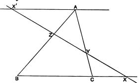
Through A draw AX' parallel to BC to cut the straight line XYZ in the point X'.
